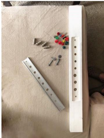
At present, this pass-through system has 4 SO-239 barrels, two binding posts for balanced feedline, a BNC pass-through (with a SMA adapter), and a good ground from the aluminum plate.
