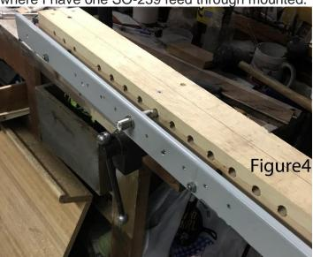
When I was satisfied, I drilled and mounted the rest of the SO-239s. I also wanted to mount a Cinch-Jones plug for the rotor control. So, I machined (by hand) a rectangular hole for the Cinch-Jones plug for the rotor cable.
