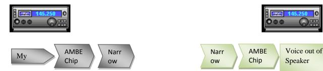
In DV (Digital Voice mode) your voice goes through the Advanced Multi-Band Excitation (AMBE) chip where it is encoded digitally plus text, and any other data, then stuffs it out the Antenna as Narrow FM.
