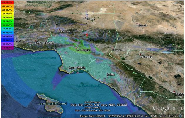
K6CPT Coverage Estimate @ 145.300 MHz, with approximations for ERP and antenna structure height, out to 113 km radius
