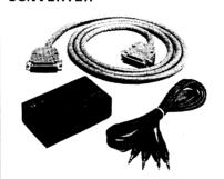
For remote transceiver control using a personal computer equipped with an RS-232C output port. You can change operating frequencies, memory channels, etc., with your computer keyboard.
