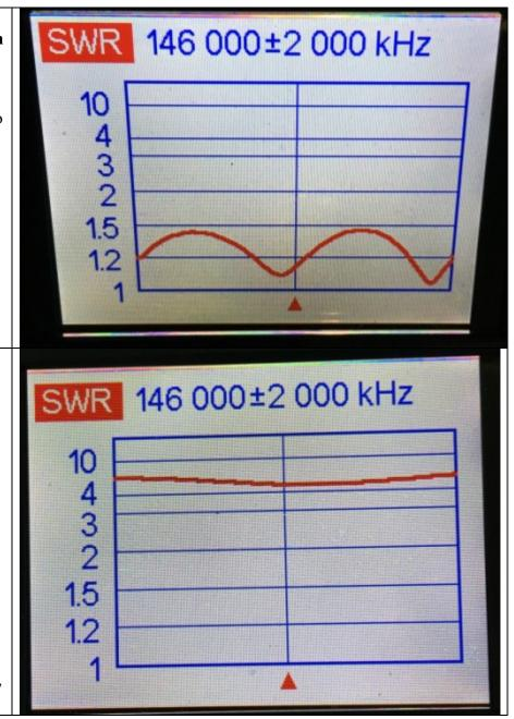
Duplexer connected to the feedlines from Position 2 ICOM 2200H 2m single band radio and the Position 3 Alinco DR 235 220 single band radio. Each radio should have its own feedline and single band antenna. This duplexer is now superfluous.
