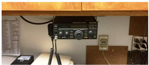
**Measurement Results:** On 6 meters the radio experienced 20dB over 9 noise level; power output was 10w however full power functions normally on 10M. Coax #5 is connected to a good 6 meter antenna; SWR @ 51.50 MHz 1.5:1. There is a tuner cable connected for the outboard tuner but that function does not work.
