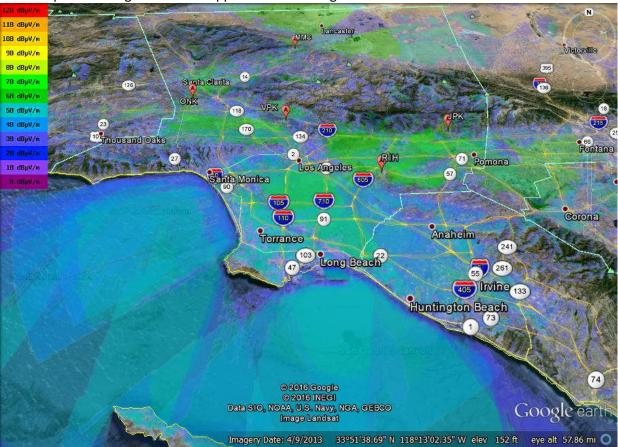
Transmitting from the Rolling Hills Rx site would start to fill uncovered areas in Palos Verdes, the Beach Cities at the coast and Malibu. There should be 3 new duplexers in the pipe line. We would like to get the Rolling Hills Rx site transmitter going as soon as possible.
