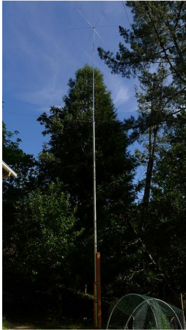
60' Top Loaded Vertical, 160/80M. Great on 30 and 17M.
