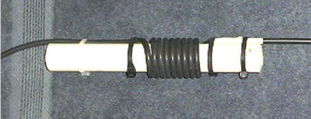
No drilling of the PVC pipe necessary for this version.
