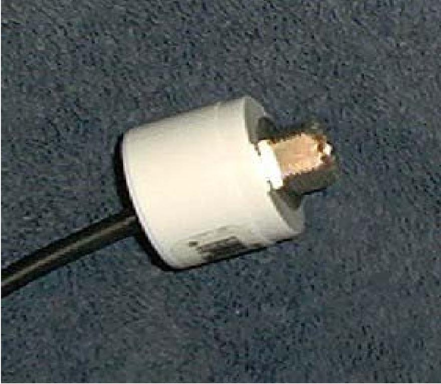
Mount the SO239 in the pipe cap and tighten the mounting nut.
