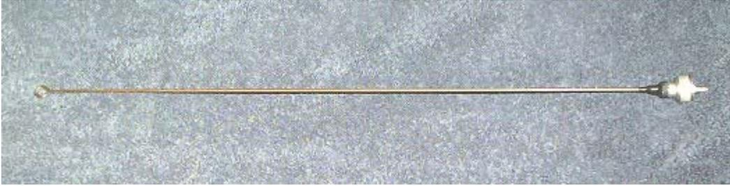
Solder a 20 inch piece of welding rod or any stiff wire (coat hanger) to the center of a PL259. Set up the antenna about 5 feet off of the ground and trim the top of the wire until your lowest SWR is around 146.500. You should have no problem getting it down to 1.2:1 with SWR no higher than 1.5:1 across the entire 2 meter band. Fill the hole in the top of the PL259 with hot glue, silicone, or liquid electrical tape.
