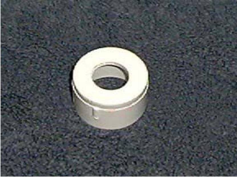
Prepare a  $\frac{3}{4}$  inch pipe cap by drilling a hole in the center of the cap. The hole should be large enough to snugly mount the SO239.
