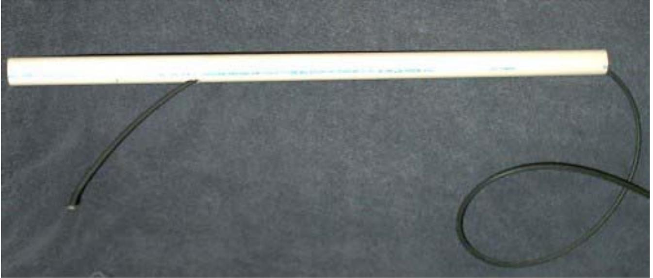
Thread the free end of the RG58 coax through the top of the pipe and bring it out of the hole you drilled at the 16 inch mark. Actually it would be easier to thread the coax through the hole and out the top *before* you solder the SO239 on the coax. Either way will work.
