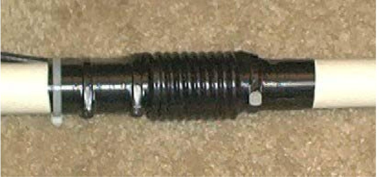
The choke may be covered, secured and weather proofed two ways.
