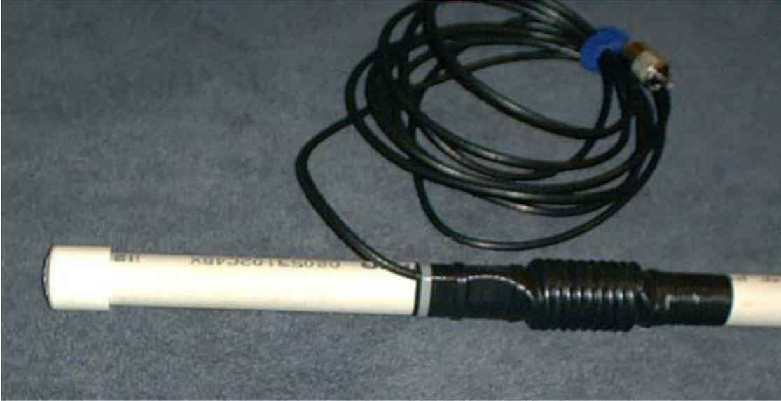
**A PVC pipe cap keeps the whip inside.**
