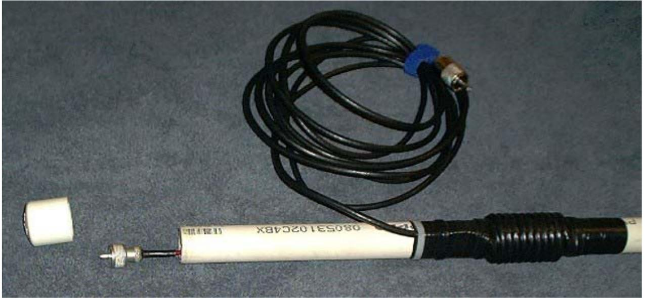
**The whip slips neatly into the base for storage.**
