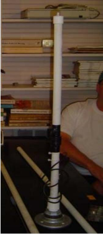
Finished antenna bottom section on a pipe flange stand.
