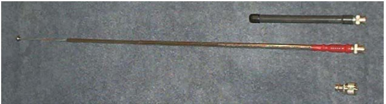
With a BNC adapter you may use any HT antenna on top of the resonant shield base. The telescoping 5/8 wave antenna will give you some gain. The rubber duck will work better on the resonant shield base than it does on the HT but it will still radiate like a dummy load. Maybe more like a leaky dummy load.
