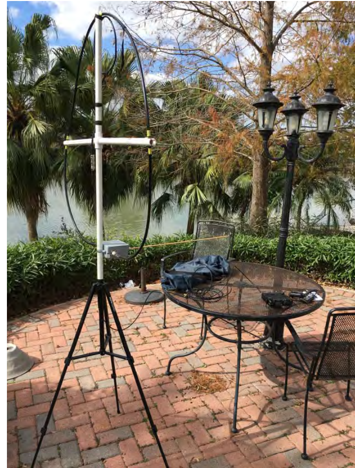
Antenna deployed for 40m thru 15m and directly connected to FT-817ND
