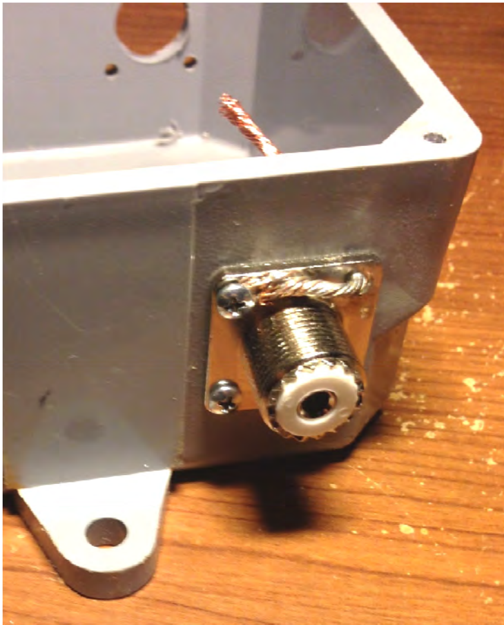
Install UHF Panel mount Connectors with connection to Solder braid
