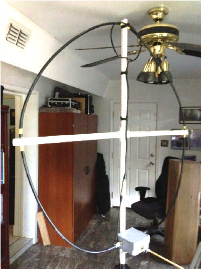
Antenna configured for 40m thru 15m
