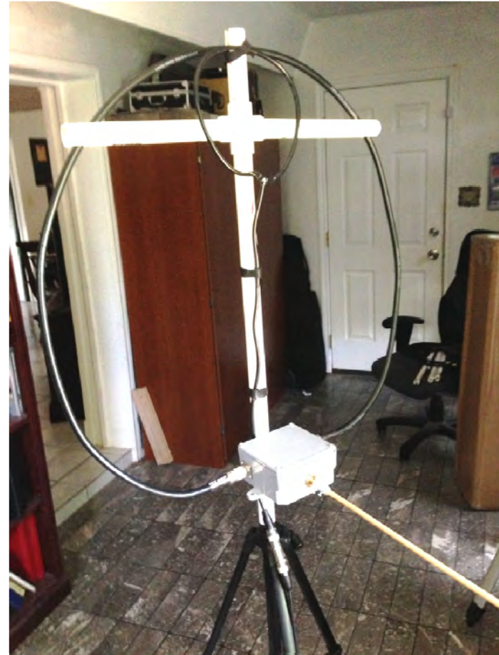
Antenna configured for 15m thru 10m • Note smaller arms for smaller loop
