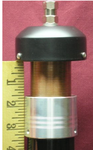
Model 300A -- 7.1 MHz with 5 ft. whip and 1 1/2" of coil showing
