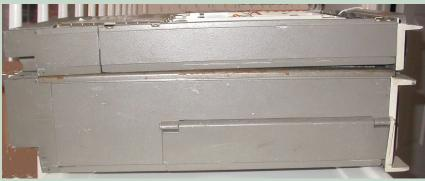
There are two versions. The standard (shown on top) and the 'E' Extended series (shown on the bottom) that is double height. The E-series allowed inclusion of a 2<sup>nd</sup> receiver. This may be removed and a ham Repeater controller and small mobile duplexer inserted.
