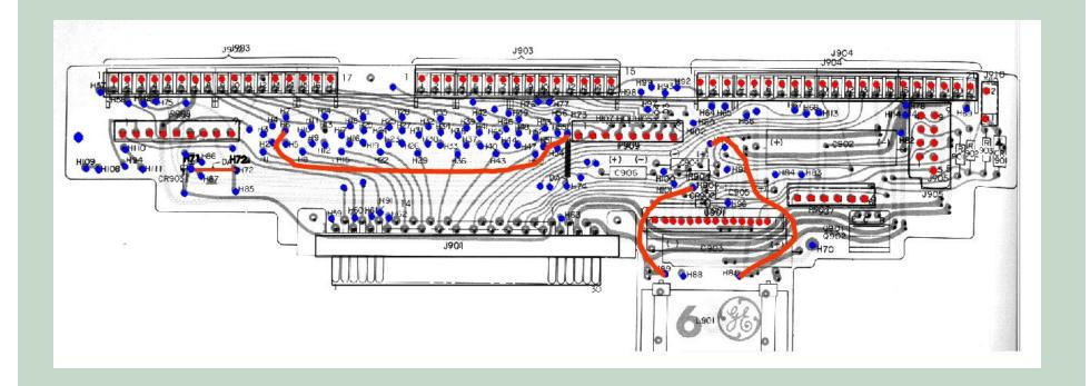
Only four added wires and one cut necessary to modify a simplex mobile radio into a full duplex repeater.
