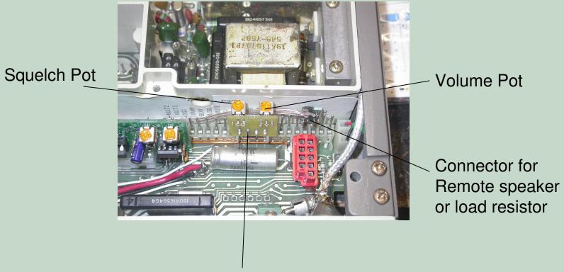
Since the radio does not have the original control head, you Must provide a volume and squelch pot. NHRC makes a nice plug in board.
