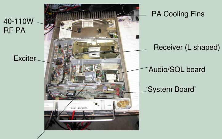
Connections for an external controller can be made on Sys board Molex connectors. A vol and sql pot must be added to replace the original front mount control head.
