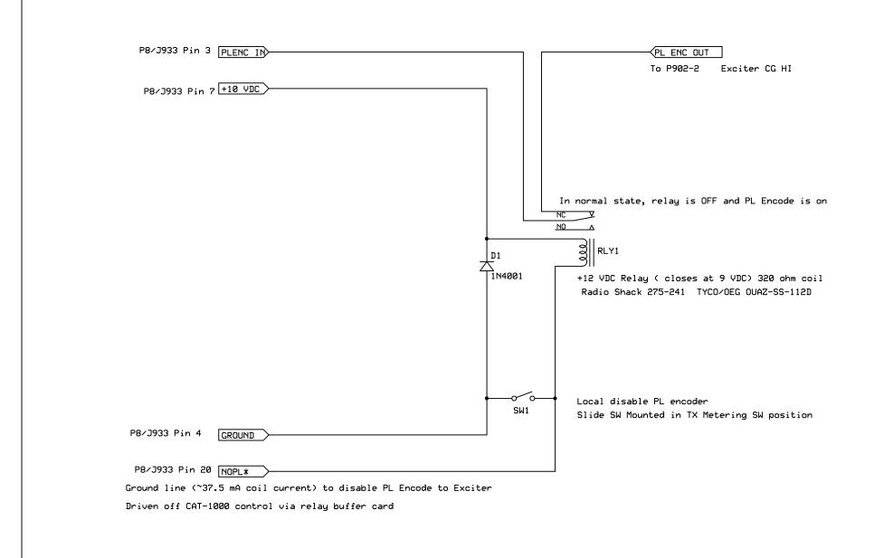
Remove wire going to P8 pin 3 and insert the relay contact in series with audio line P8 pin 20 unused in non-metering panel GE M II base/repeaters
