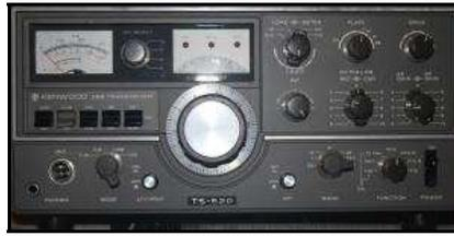
and CW modes in the 80 through 10 meter ham bands. It also features receive of WWV at 10 MHz. The TS-520 features a very accurate linear analog display dial. Power input is 120W PEP SSB and 100W CW. (This transceiver does not have general coverage receive). The hybrid circuit includes three 6146A and two 12BY7A tubes plus 1 IC, 17 FETS, 45 transistors and 84 diodes. **REDUCED \$185 or best offer. Contact W4JNC, president @ w4amc.com.** (Phone 758-1244)
