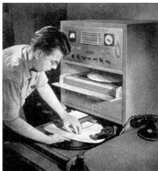
Figure 112: Flexible disk recorders used to record unknown signals for further analysis.
