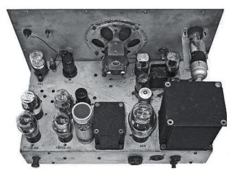
Figure 18: Interior view of the aperiodic receiver.
