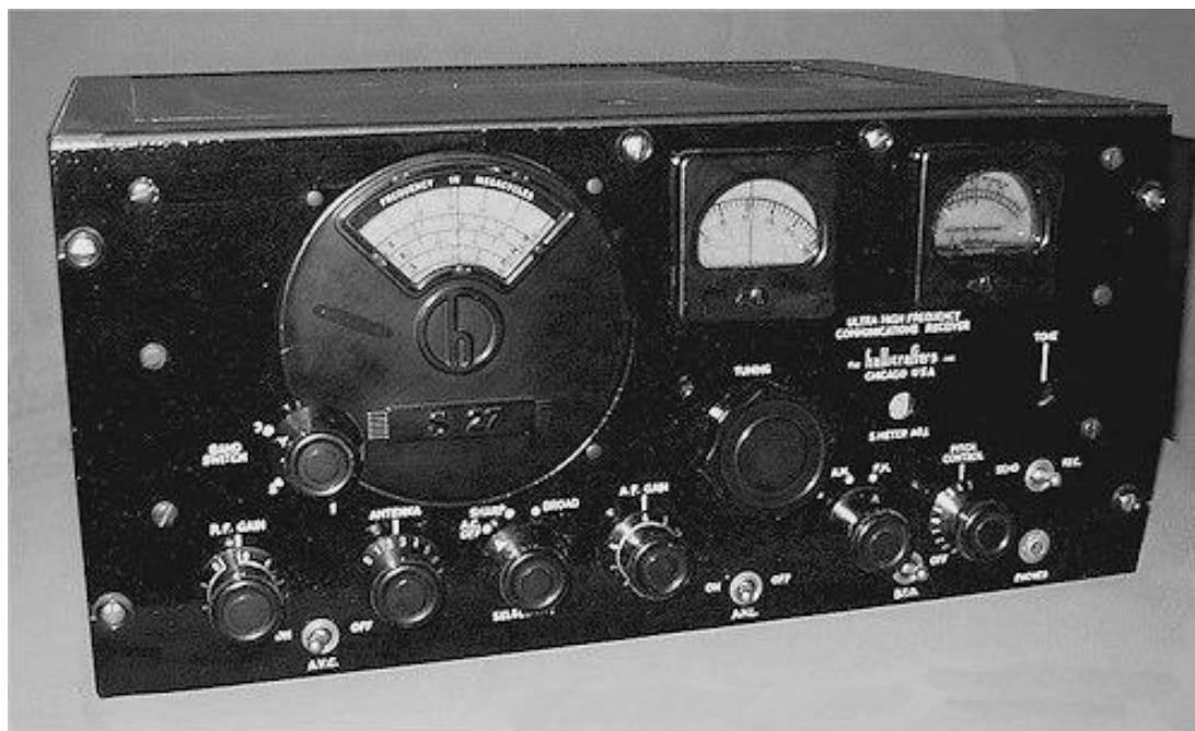
Figure 10: Hallicrafters S-27 receiver used at RID monitoring stations and in mobile units.
