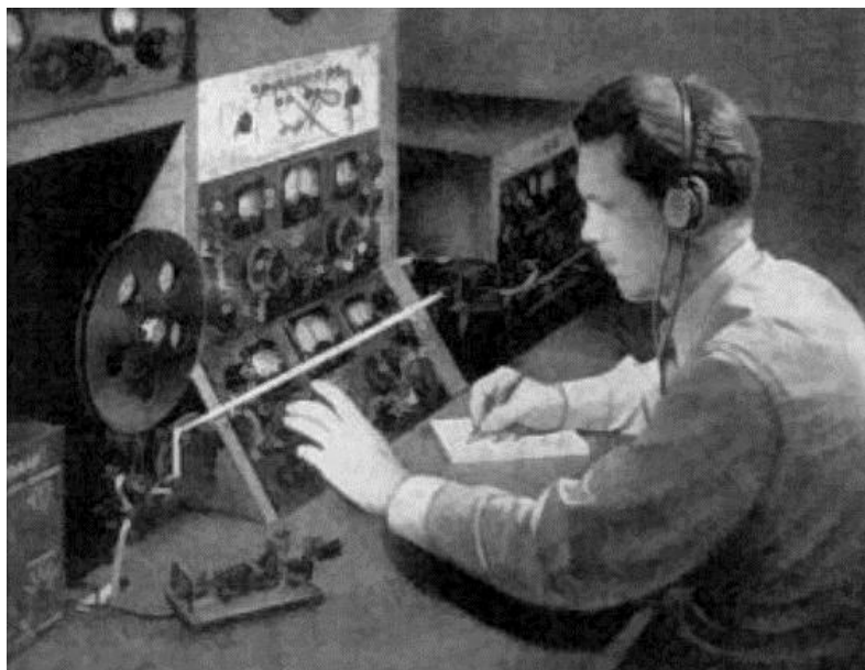
Figure 29: William J. Hoffert (W5HVB) recording high speed code on a Boehme tape machine.
