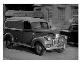
Figure 96: RID Mobile Unit with concealed loop antenna.
