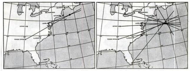
Figure 54: Bearings taken from monitoring stations covering a wide range of angles give the highest accuracy fix.
