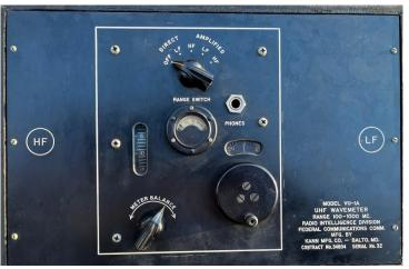
Figure 19: UHF Wavemeter manufactured by Manuel Kann
