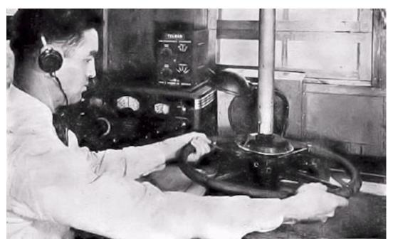
**Figure 49:** Assistant Supervisor K.W. Miller, W5AOC, taking a bearing with an Adcock direction finder. The antenna was rotated to obtain a null in signal strength. At this point the antenna is broadside to the direction of arrival of the signal. You can see the sideband slicer sitting on top of the SX-28.
