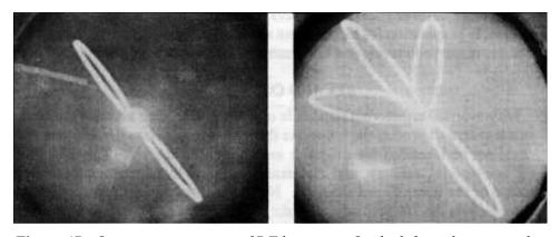
**Figure 47:** O-scope presentation of DF bearings. On the left is a bearing with a tight figure eight pattern. On the right is a bearing showing the sense of the direction of the arriving signal.
