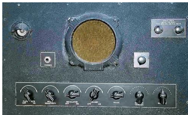
Figure 14: Aperiodic receiver developed by RID.
