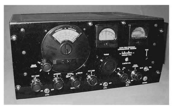
Figure 10: Hallicrafters S-27 receiver used at RID monitoring stations and in mobile units.
