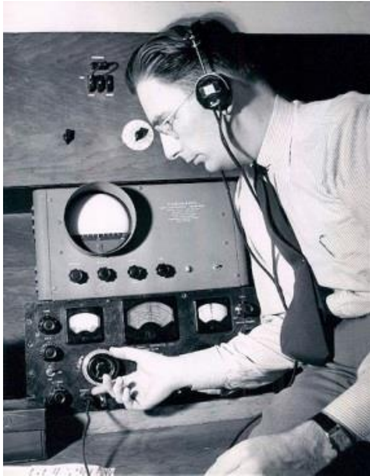
Figure 92: Dr. Marcel Wallace (F3HM) inventor of the panoramic display 1932. Shown here with a Panoramic SA-1 T-100 panadapter connected to a Hallicrafters SX-28.
