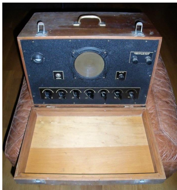
Figure 15: SSR-201 Aperiodic Receiver manufactured for RID and OSS. This one belongs to Brian Harrison, KN4R.
