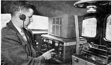
**Figure 100:** RID prowl car interior. The operator (Ed Atems) tunes in a signal on the Hallicrafters SX-28 while the signal is being recorded on a Telecord wax cylinder recorder. The loop did not show while the car was cruising but only when taking a bearing. Other receivers in the car covered 75Kc to 300 Mc.
