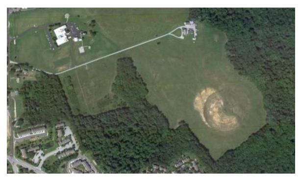
**Figure 180:** Aerial view of Laurel monitoring station circa 2010. The building in the upper left corner is the laboratory. The monitoring station is the building top center and the remnants of the Wullenweber DF antenna can be seen on the lower right.
