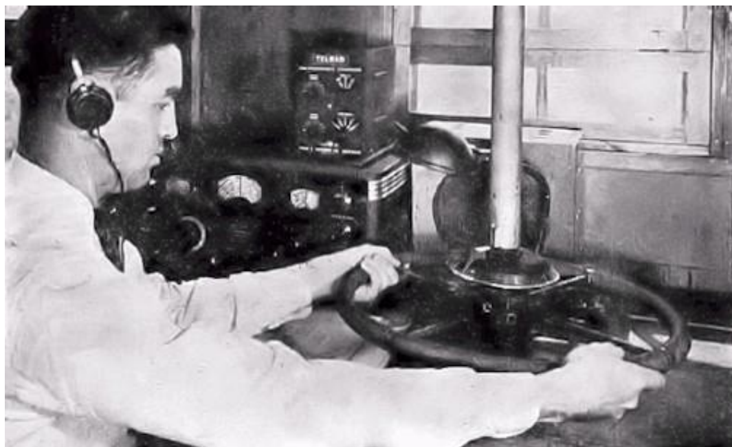
Figure 43: Assistant Supervisor K.W. Miller, W5AOC, taking a bearing with an Adcock direction finder. The antenna was rotated to obtain a null in signal strength. At this point the antenna is broadside to the direction of arrival of the signal. You can see the sideband slicer sitting on top of the SX-28.
