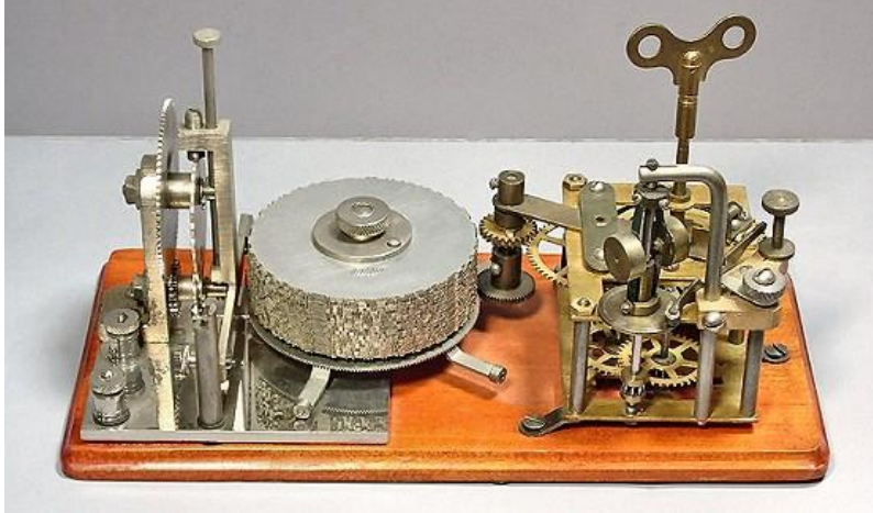
Figure 35: Omnigraph - used by FCC examiners to give morse code examinations during the 1910s and 1920s.
