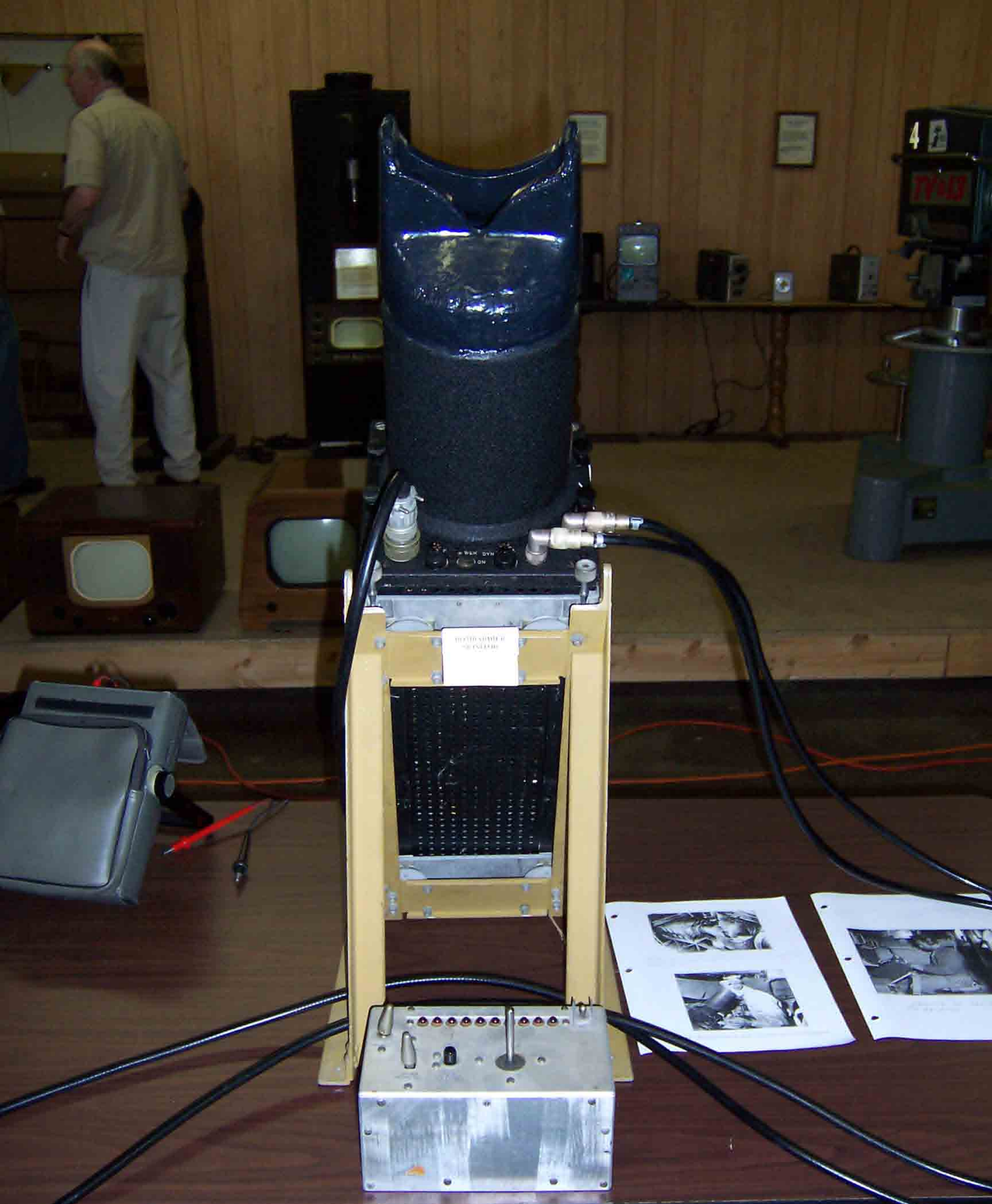
Bombardier Repeat monitor driven from the receiver. The joy stick box would control the bomb to the target
