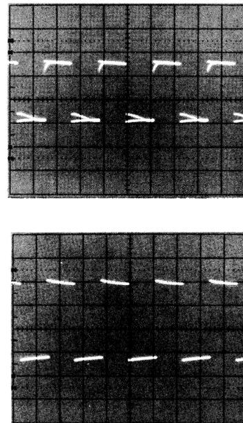
**Figure 28.** DIFFERENTIAL MEASUREMENTS allow you to remove unwanted information from a signal anytime you have another signal that closely resembles the unwanted components. For example, the first photo shows a 1 kHz square wave contaminated by a 60 Hz sine wave. Once the common-mode component (the sine wave) is input to channel 2 and that channel is inverted, the signals can be added with the ADD vertical mode. The result is shown in the second photo.
