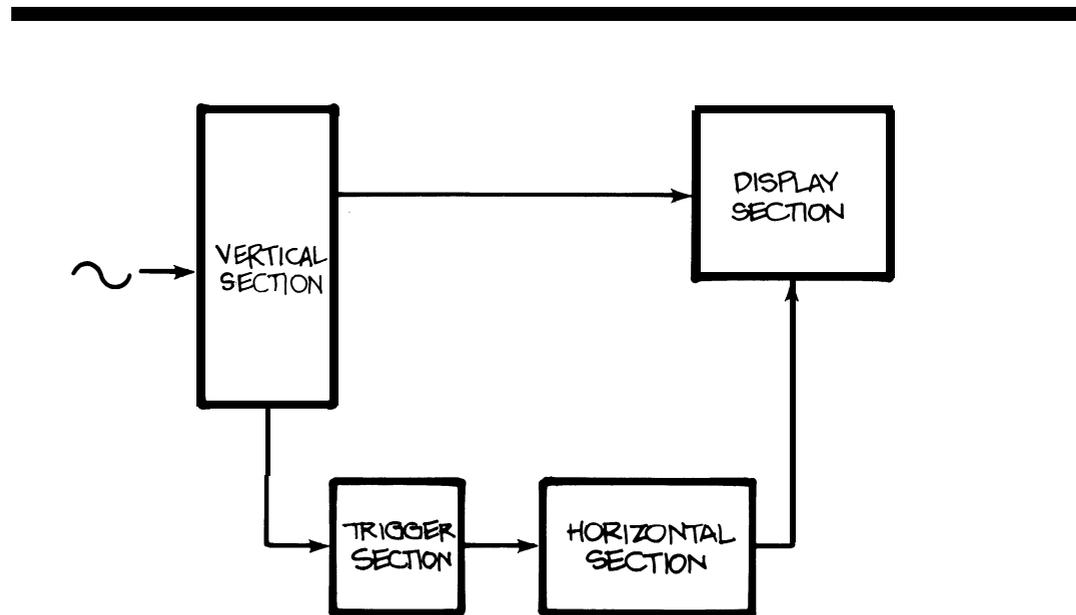
**Figure 1.** THE BASIC OSCILLOSCOPE in its most general form has only four functional blocks: vertical, horizontal, trigger, and display systems (and sometimes, sections). The display system is also sometimes called the CRT (for cathode-ray tube) section.
