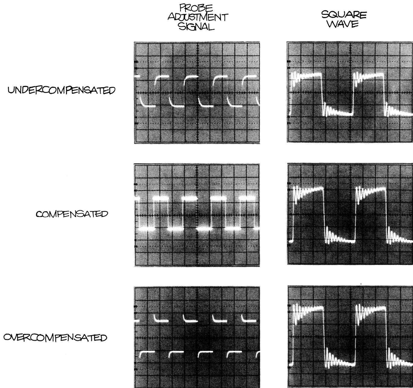
**Figure 23.** IMPROPERLY COMPENSATED PROBES can distort the waveforms you see on the screen of your scope. In the photographs the probe adjustment signal and a 1 MHz square wave are shown as they will appear with proper and improper compensations. Notice the amplitude and ringing changes on the square wave with the differences in compensation.
