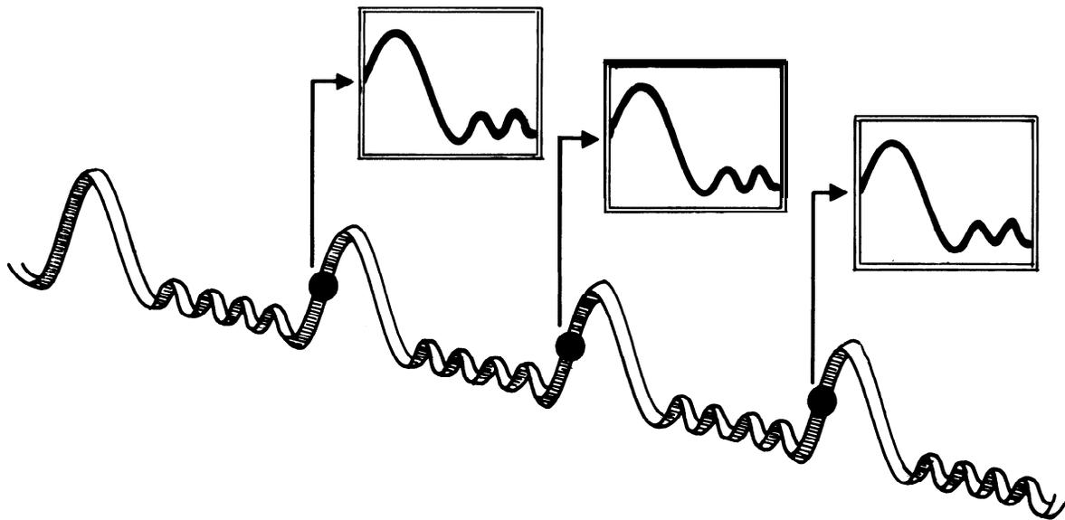
**Figure 9.** TRIGGERING GIVES YOU A STABLE DISPLAY because the same trigger point starts the sweep each time. Slope and level controls define the trigger points on the trigger signal. When you look at a waveform on the screen, you're seeing all those sweeps overlaid into what appears to be one picture.
