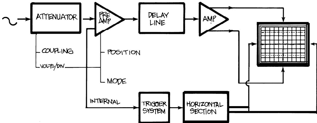
**Figure 4.** THE VERTICAL SYSTEM of a Tektronix 2200 Series scope consists of two identical channels though only one is shown in the drawing. Each channel has circuits to couple an input signal to that channel, attenuate (reduce) the input signal when necessary, preamplify it, delay it, and finally amplify the signal for use by the display system. The delay line lets you see the beginning of a waveform even when the scope is triggering on it.
