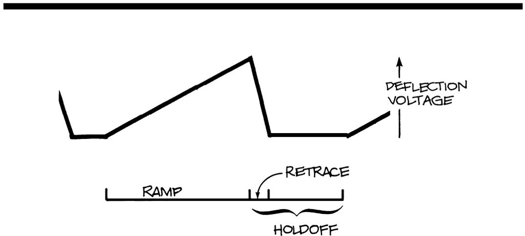
**Figure 7.** THE SAWTOOTH WAVEFORM is a voltage ramp produced by the sweep generator. The rising portion of the waveform is called the *ramp*; the falling edge is the *retrace*; and the time between ramps is the *holdoff* time. The sweep of the electron beam across the screen of a scope is controlled by the ramp and the return of the beam to the left side of the screen takes place during the retrace.
