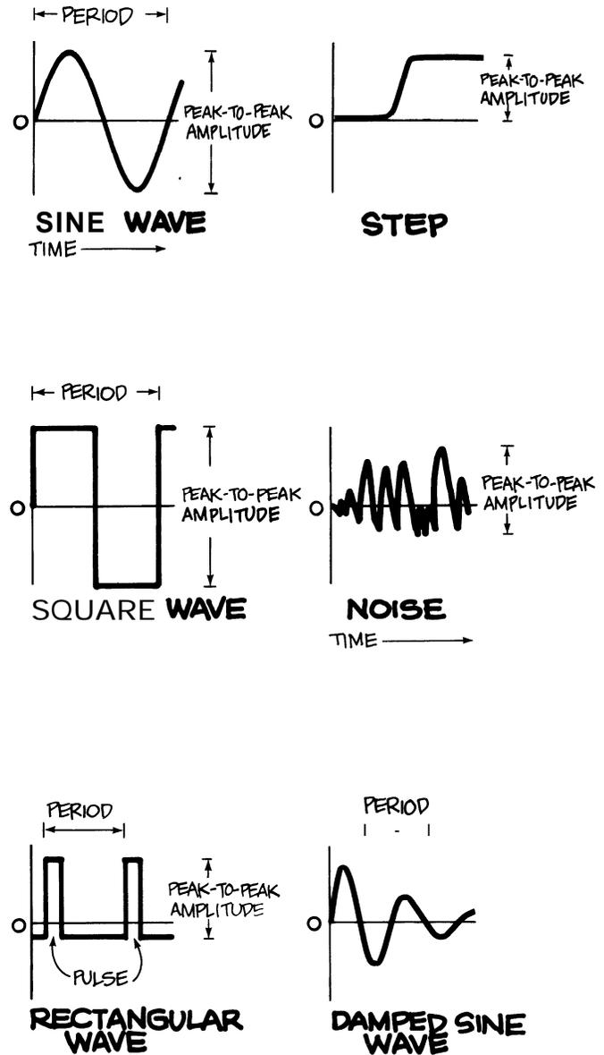
**Figure 18.** PERIOD IS THE TIME REQUIRED FOR ONE CYCLE OF A SIGNAL if the signal repeats itself. Period is a parameter whether the signal is symmetrically shaped like the sine and square waves above, or whether it has a more complex and asymmetrical shape like the rectangular wave and damped sine wave. Period is always expressed in units of time. Naturally, one-time signals like the step or uncorrelated signals (without a time relation) like noise have no period.
