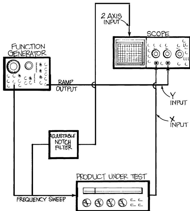
**Figure 29.** USING THE Z-AXIS can provide additional information on the scope screen. In the set-up drawn above, a function generator sweeps through the frequencies of interest during the product testing—20 to 20,000 Hz, in this case. Then an adjustable notch filter is used to generate a marker, at 15 kHz, for instance, and this signal is applied to the Z-axis input to brighten the trace. This allows the tester to evaluate the product's performance with a glance.
