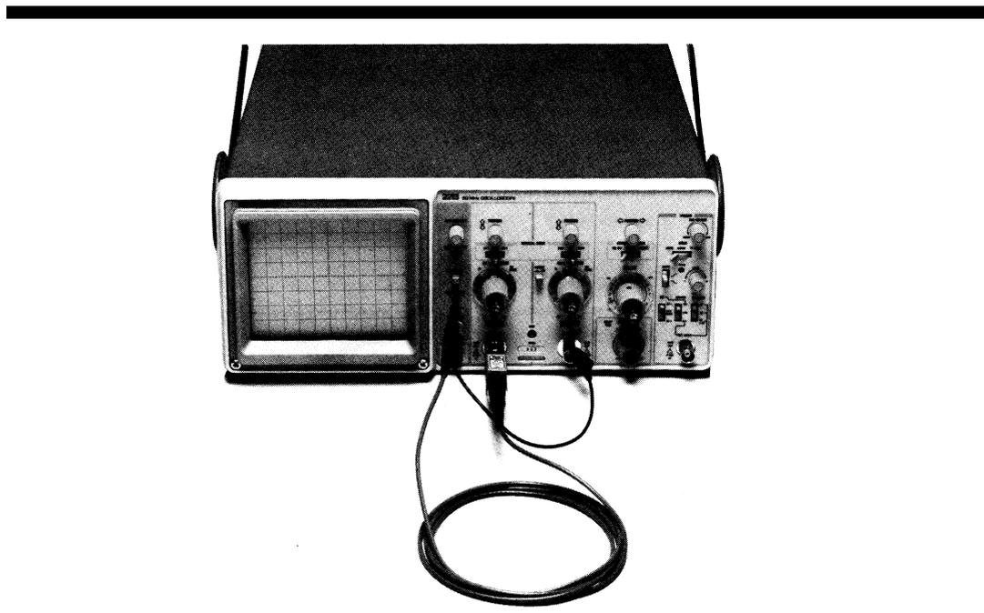
**Figure 6.** THE TEKTRONIX P6120 10X PROBE connects to the BNC connector of either channel 1 (shown) or 2; unlike the photo, the probe's ground strap is usually connected to the ground of the circuit you are working on. The probe adjustment jack is labeled PROBE ADJUST and is located near the CRT controls on the front panel.
