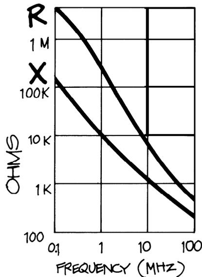
**Figure 15.** PROBE IMPEDANCE IS RELATED TO FREQUENCY as shown in the table above. The curves plot both resistance (R) and reactance (X) in ohms against frequency in megahertz. The plot shown is for the Tektronix P6120 probe on a I-meter cable.
