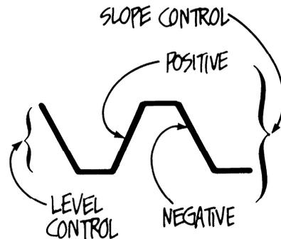
**Figure 10.** SLOPE AND LEVEL CONTROLS determine where on the trigger signal the trigger actually occurs. The SLOPE control specifies either a positive (also called the *rising* or positive-going) edge or on a negative (*falling* or *negative-going*) edge. The LEVEL control allows you to pick where on the selected edge the trigger event will take place.
