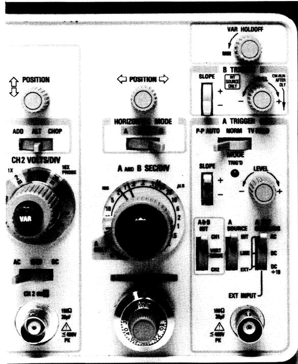
**Figure 30.** THE DELAYED SWEEP CONTROLS of the dual time base 2215 are shown on the photograph above. They include: HORIZONTAL MODE (under the horizontal POSITION control); B TRIGGER SLOPE and LEVEL; ALT SWP SEP (alternate sweep separation, between the two vertical POSITION controls — not shown), and a concentric A and B SEC/DIV control. The B DELAY TIME POSITION dial is at the bottom of the column of horizontal system controls.
