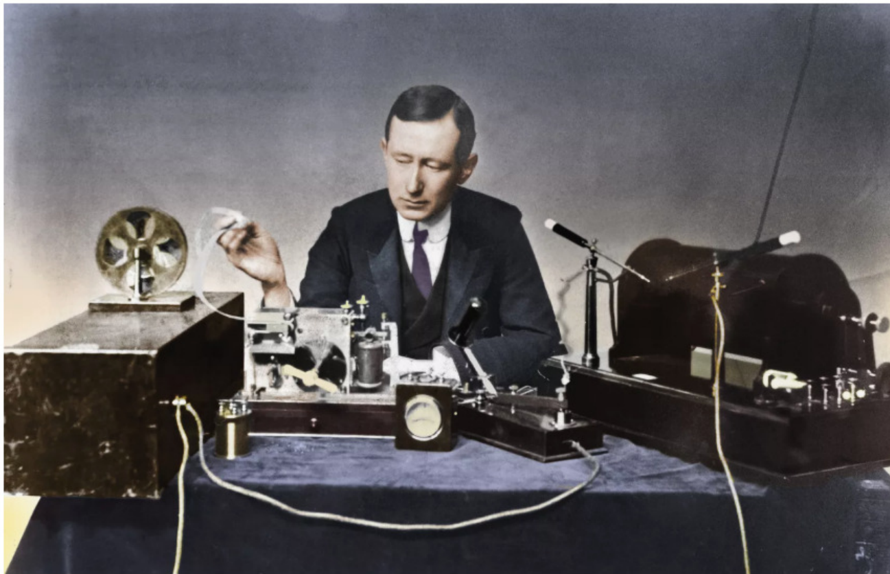
📷 Marconi with typical apparatus, including 10-inch induction coil spark transmitter (right), morse inker and grasshopper key in center. Print Collector / Getty Images
