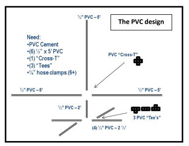
on my back deck, I drew up a quick prototype of a self-standing ground-plane – see the basic design of the PVC tubing in the figure to the right.
