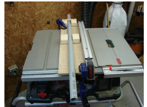
Figure 11 – My HB conduit splitter
