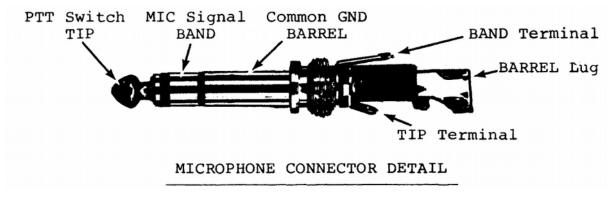
Since the crystal 4 pole filter system is common to both receiver and transmitter circuits, audio signals picked up by the microphone while receiving may be applied to the audio receiver system, causing possible acoustic howl or reverberation. To completely eliminate this in the PTT mode of switching, it is recommended that a SPDT type switch be used in the microphone and that the microphone signal lead be shorted to ground during receive.
