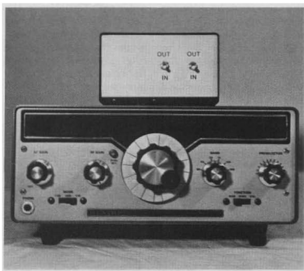
Photo B. Front view of modified HR-1680 (with completed filter-blanker on top) shows details of modified spinner knob.
