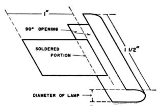
inches long and solder it to the shield leaving 1 inch free and pointing in the direction of the open slot in the shield. Paint the inside of the shield white and the outside gloss black.
