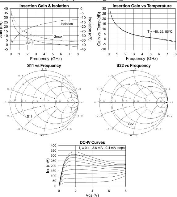
Note: S-parameters are de-embedded to the device leads. The data represents typical performace of the device. Measured s-parameter data files can be downloaded using a link found on the SGA-9189 device page from our web site at www.stanfordmicro.com.
