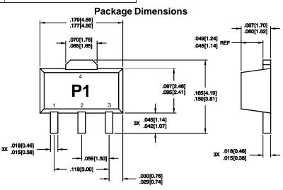
Pin assignments shown for reference only, not marked on part
