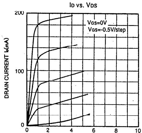
DRAIN TO SOURCE VOLTAGE V<sub>ds</sub>(V)
