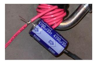
Wrap the coils in electrical tape and close the quick link. About 1.5" from the right end of the inductor strip 1/4" of insulation off the red wire and solder in the + lead of the capacitor. Make sure you observe the capacitor polarity. In the picture you can see the negative arrow on the capacitor pointing down. Solder the 18" piece of black wire to the negative lead of the capacitor. (Above)
