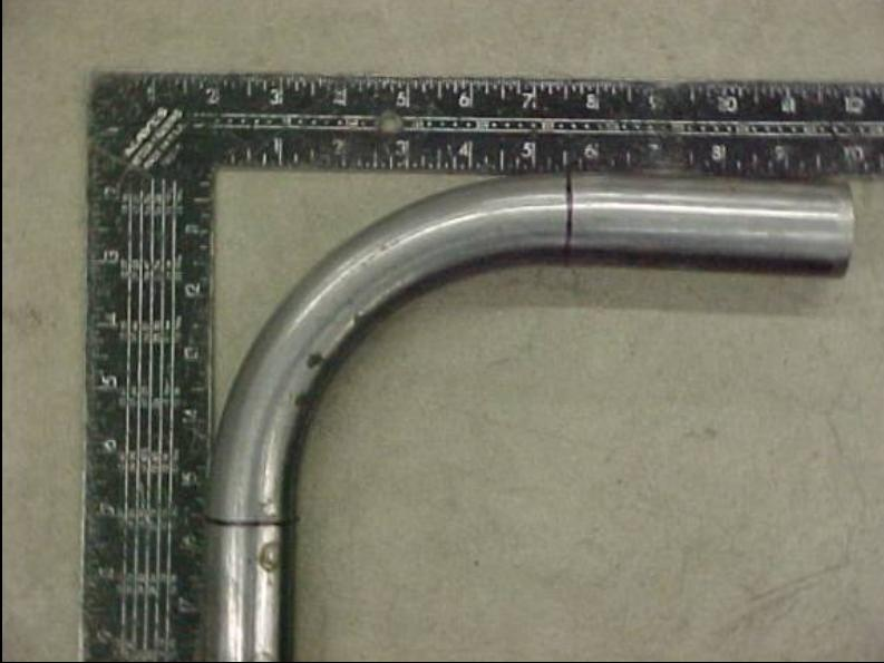
Lay your 90 inside your square and see how many inches that it takes to complete the bend, start to stop. They both should be the same measurement, in this case it's  $5 \frac{1}{2}$ ". See, by doing it this way, you're not worried about what the centerline is or what size tube it is or any of that other "fancy" stuff. You KNOW that it takes  $5 \frac{1}{2}$ " to complete a bend.
