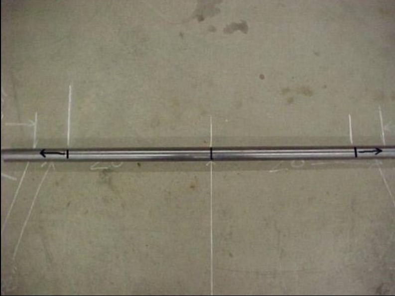
Chalk up your tube in the bender by lining up the marks and the direction arrow (seam to the inside).
