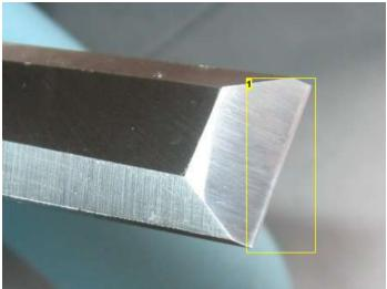
**Image Notes** 1. There it is - that little thin line is a second bevel, which alone needs to be sharpened when your chisel starts getting dull.
