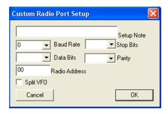
If a particular radio model supports CPP selection, then an appropriate Baud Rate along with Stop Bits, Data Bits and Parity can be entered, whenever the Baud Rate is 0, the coded default parameters are used. Changing the baud rate to other than 0 requires selection of all serial port parameters by the user.
