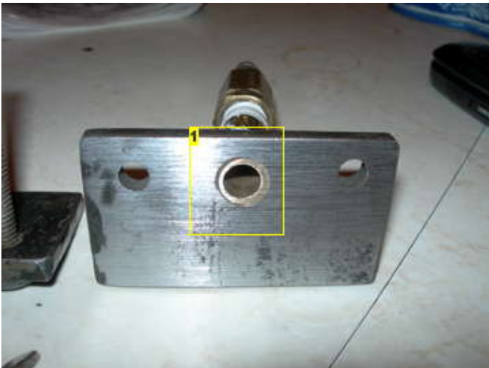
Image Notes 1. Here is where the CO2 will enter your bottle. Make it line up over the U-shape.
