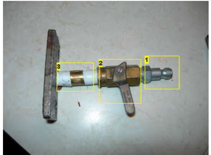
Image Notes 1. Quick release coupling 2. convenience valve 3. nipple
