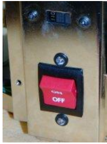
A new switch was put in the original hole and the original mounting holes drilled out for the LEDs.
