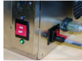
When the battery is fully charged only the green LED (connect) glows
