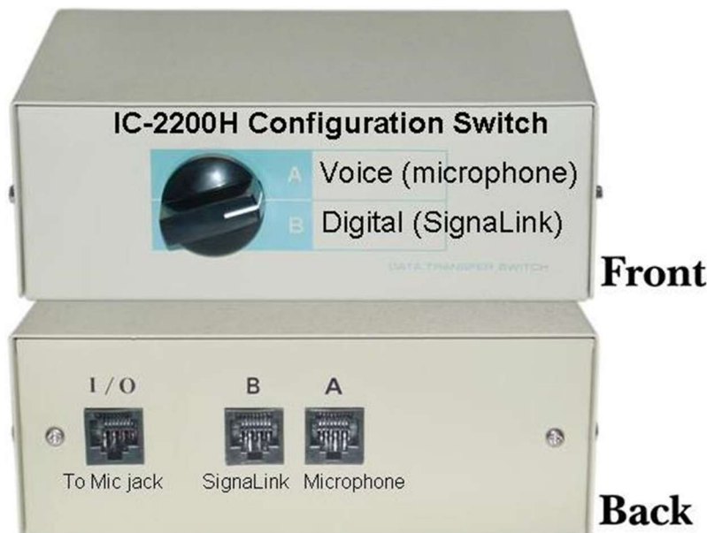
Figure A-4. Notional concept for a network switch to select either voice (microphone) operation or digital operation from the IC-2200H 2m transceiver with a simple and inexpensive RJ-45 two-position rotary switch
