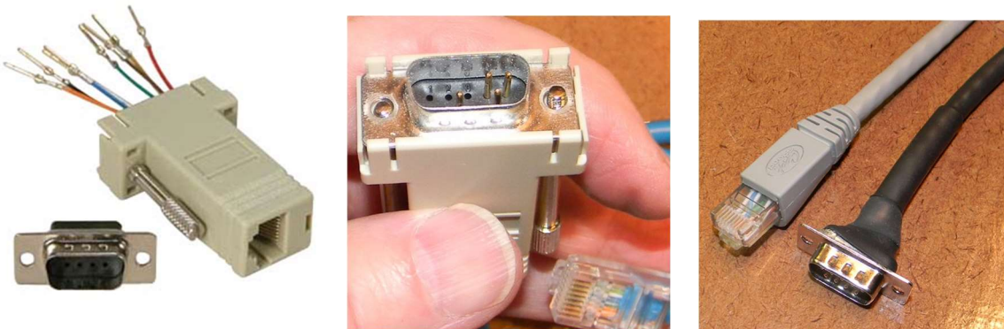
Figure 10. (Left) User-configurable DB9-male adapter; (Center) DB9 adapter wired for pins 4, 5, 7 and 9, as required for the Alinco DR-235 Signalink cable; (Right) Fabricated and labor-intensive alternative cable for Signalink RJ-45 connector to Alinco DR-235 transceiver's rear DB9 data connector. The recommended option for this application is the adapter.
