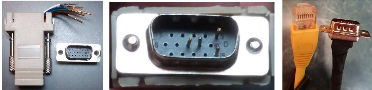
Figure 12. (Left) User-configurable HD15-to-RJ45 adapter; (Center) HD15 adapter wired for pins 5, 8, 9 and 15, as required for the Bridgecom BCM-220 SignalLink cable; protruding plastic case trimmed back to fully seat male connector on rear of radio; (Right) Fabricated and labor-intensive alternative cable for SignalLink RJ-45 connector to Bridgecom BCM-220 transceiver's rear HD15 data connector. The alternative method of direct connector-to-connector soldered cable may be employed for some DCS installations if a sufficient number of HD15-to-RJ45 adapters are not available.
