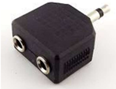
Figure A-3. Audio 3.5mm “Y” splitter plugged into the IC-2200H rear speaker jack, enabling both an external speaker and an audio cable to the Signalink rear SPKR jack to be connected
