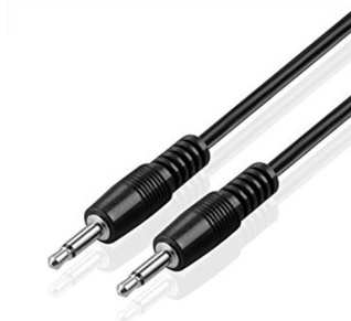
Figure A-2. Commonly available monaural cable to connect speaker jack at rear of radio to SPKR jack at rear of SignalLink USB unit (supplied with each SignalLink USB unit); this connection provides the Data Out signal that will be routed via the SignalLink unit to the computer for NBEMS digital data processing in FLDIGI
