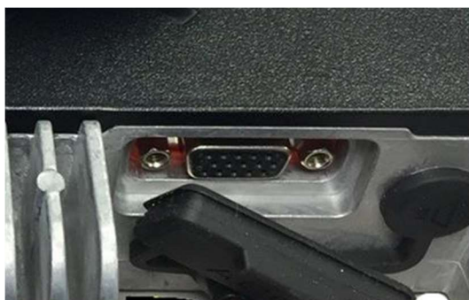
Figure 11. Rear HD15 female accessory connector with cover removed (Only pins 5, 8, 9 and 15 are of interest.)
