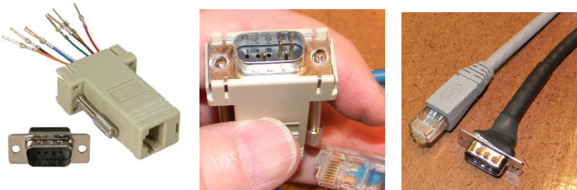
Figure 10. (Left) User-configurable DB9-male adapter; (Center) DB9 adapter wired for pins 4, 5, 7 and 9, as required for the Alinco DR-235 SignalLink cable; (Right) Labor-intensive alternative fabricated cable for SignalLink RJ-45 connector to Alinco DR-235 transceiver's rear DB9 data connector. The recommended option for this application is the adapter.
