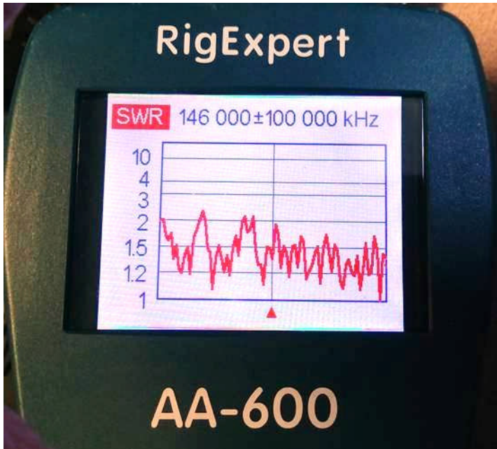
Figure 3. SWR of outside 2m antenna shows unusual behavior—generally less than 2:1 everywhere and no apparent resonance(s)
