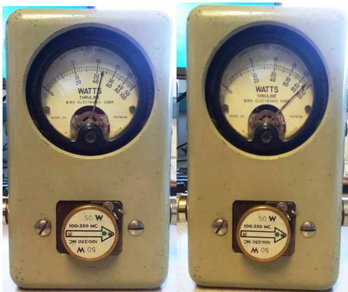
Figure 4. Left and right photos indicate, respectively, output power of ~23 watts in low-power mode, ~45 watts in high-power mode
