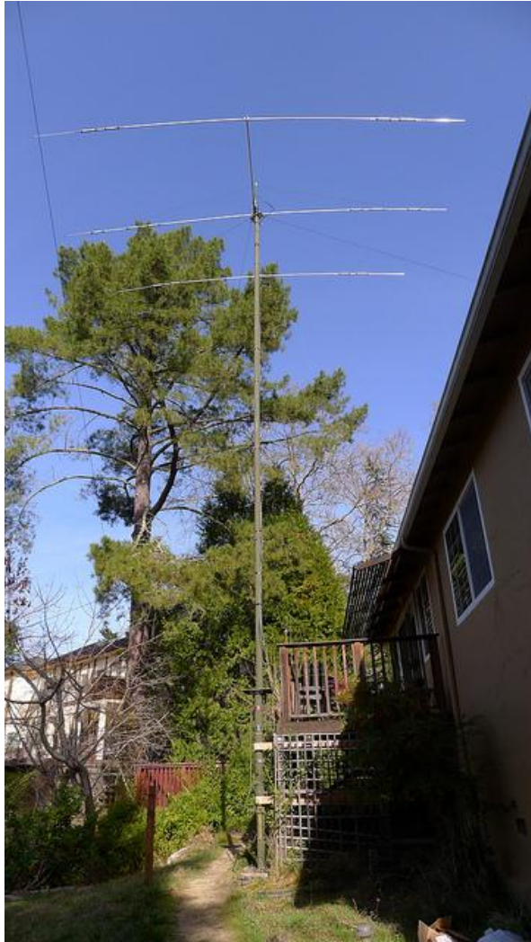
A3S + 30M at 46' on AB-952 - Replaced 20M Moxon at 30'
