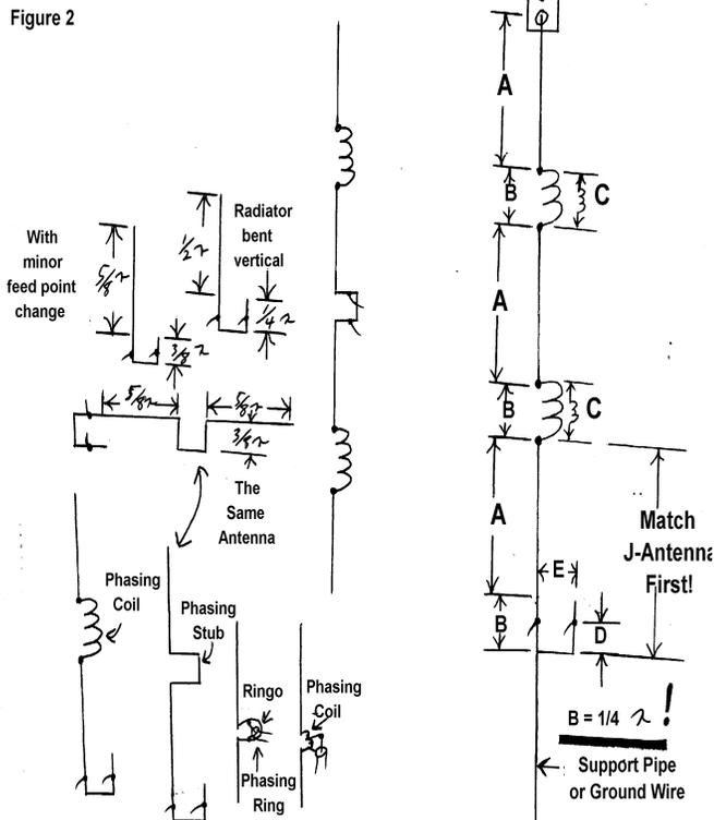
For use on two meters, the antenna is made from #12 stranded copper wire for the radiators. The loading coils (see Fig. 3) are
