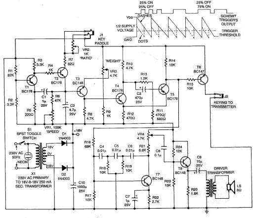
tacts, dots and dashes are formed. When the key is in open position, T1 conducts but T2 is biased off because of the conduction state of T1.
