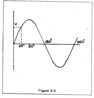
also called the effective value for a particular reason. AC current having RMS value of 230 volts will have the same effect as a DC supply of 230 volts. If we connect a heater to 230 volts RMS it will have the same heat as when connected to 230 volts DC. If we connect a bulb it will glow with the same brightness as a bulb connected to 230 volts DC What has been said about voltage applies equally to current also. For this reason instead of saying 230 volts RMS we simply say 230 volts.
