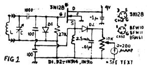
The circuit diagram of the dip meter is as shown in Fig. 1. It utilizes MOSFET 3NI28 in RF oscillator configuration (al though FET BFW 10, 11, 61 were tried with comparable success instead of 3NI28). The output of the oscillator is rectified by D2 and .01 mfd capacitor and is fed to 0-200 microampere meter through 10K linear potentiometer to adjust for a convenient level of current in the meter.
