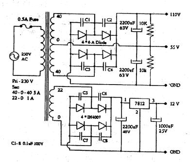
tected from high voltage transients on the AC line as well as reduce inter-carrier hum modulation of RF that may be picked up by the mains. Always use fuse in 120 V supply line. This can avoid hand full of burned IRF. It also protects the power supply itself. My final consumes around 1 A at peak. I used to 0.5 A fuse; it won't go QRT with 1 A peak current. It is better to use a fuse that can just withstand the peak current.
