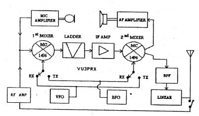
Presently the circuit is only for 7 MHz SSB operation. It can be modified for other bands by suitably changing VFO, transmit band pass filter and receiver band pass filter. I had avoided CW and AM provision for simplicity. CW and AM can be implemented by making some carrier to leak through balanced modulator. This can be done by offsetting balanced modulator by applying some external voltage to pin 4 of MC1496.
