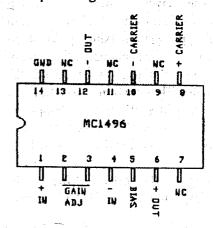
Pin 1 and pin 4 are balanced low-level inputs. Pin 8 and pin 10 are balanced high-level inputs. Pin 6 and pin 12 are outputs. Pin 5 is bias usually connected to Vcc through a resistor (normally 10k). Pin 2 and pin 3 determines gain of the mixer. The gain will be maximum when pin 2 and pin 3 are shorted. Gain can be adjusted by connecting some resistance between pin 2 and pin 3. Pin 7, pin 9, and pin 11 and pin 13 are not used.
