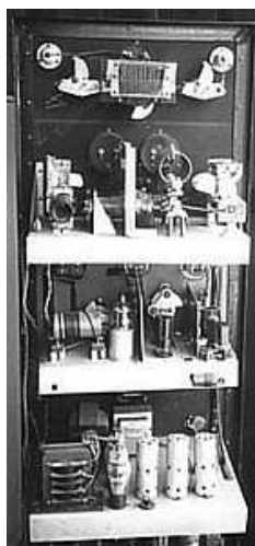
Figure 10 Modulator and RF units at VK5BR.
