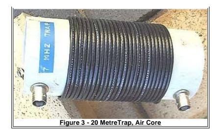
With continuous power of 50 watts fed to the antenna, a slight warming of the choke was evident.
