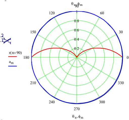
180 degrees phase shift and mode ratio B/A = 1.875 gives directivity gain = 10.03dBi = 4.87dBQ along the horizon.
