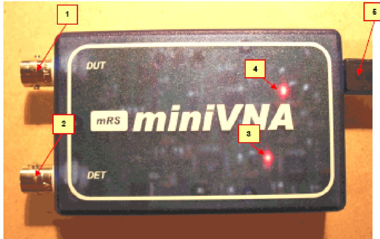
1. BNC DUT: rf out / antenna. **WARNING! Do not connect to RF transmitter**
