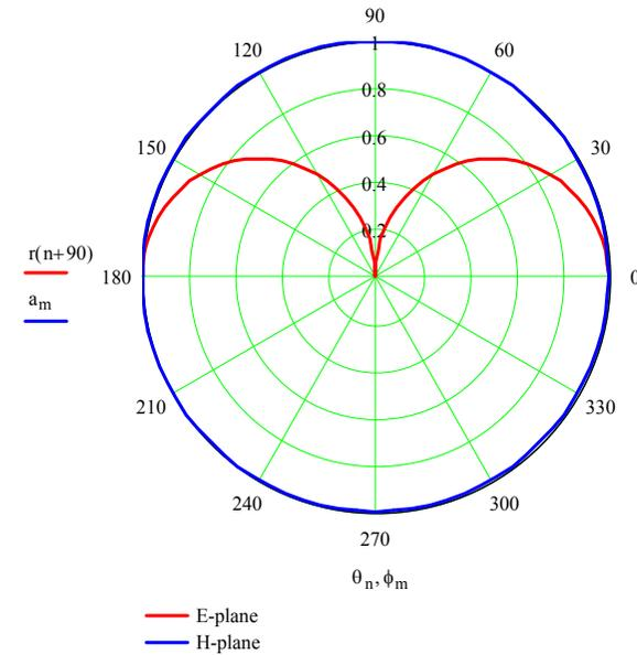
CFA D-plate radiation pattern.
