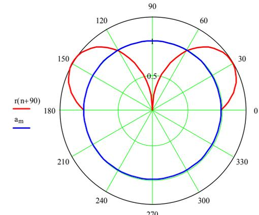
Modes 180° out-of-phase and with equal power gives directivity = 8.62dBi = 3.46dBQ along the horizon.
