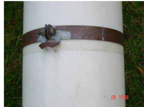
**Arno Venus 160 EH Dipole:** copper ‘tuning band’ shorted turn temperature increased from 13°C to 25°C using a non-contact thermometer (centre picture) after 15 minutes of 80 watts input to antenna. Rough estimate of no worse than 50% antenna efficiency from this. Needs more refinement.
