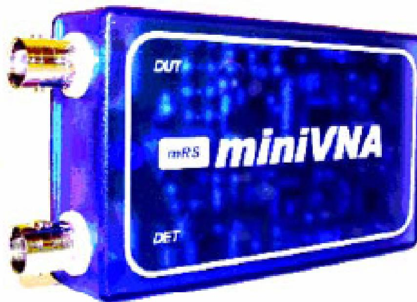
The device is designed to measure antenna impedance and filters over the HF and VHF frequency range. The small hardware (9x5.5x3cm) uses an USB connection to a PC where the antenna parameters can be displayed, one full scan takes about 0.5 sec per 500 samples, the instrument will give a big help to tune and design antennas especially for radio amateurs.
