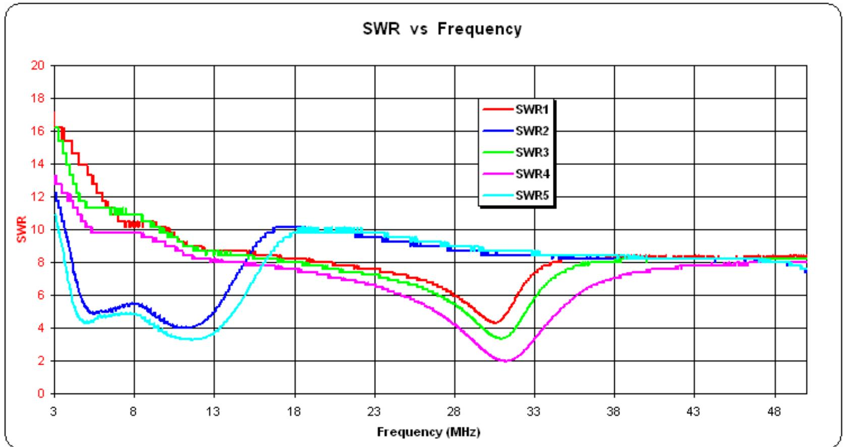
**Figure 24: Two sets of comparisons over wet clay ground.** The lower curves on the left were for a three turn loop. Those curves that are lower on the right were for a single turn with the two turns shorted. SWR 2 and 3 are for the three turn loop vertical and horizontal on the ground respectively. SWR4, 5 and 1 are for the one turn loop vertical and horizontal on the ground and then horizontal and raised 30cm above ground, respectively
