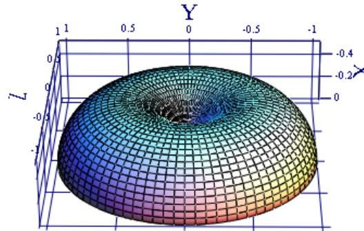
Antenna 3D Plot (E field is vertical)
