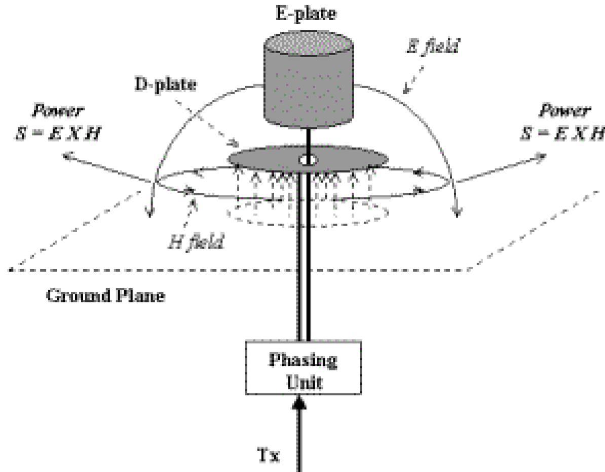
The fundamental principle underpinning CFA design is that electric and magnetic fields are produced from separate field stimuli, or field electrodes, and crossed-stressed in-phase within a small volume, called the *interaction zone*, close to the CFA structure.
