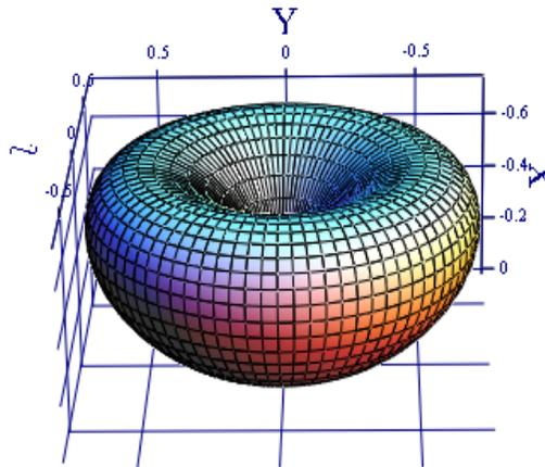
Antenna 3D Plot (E field is vertical)
