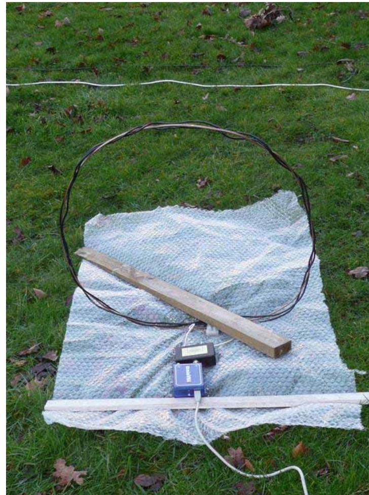
**Principle:** Loop SWR or Rho ( $\Gamma$ ) is plotted by a miniVNA in a sub-range of frequencies in the 2 to 50MHz region or around selected spot frequencies for the loop horizontally and vertically on the ground, The values for ground permittivity and conductivity are extracted *heuristically* from the differences between the plots.
