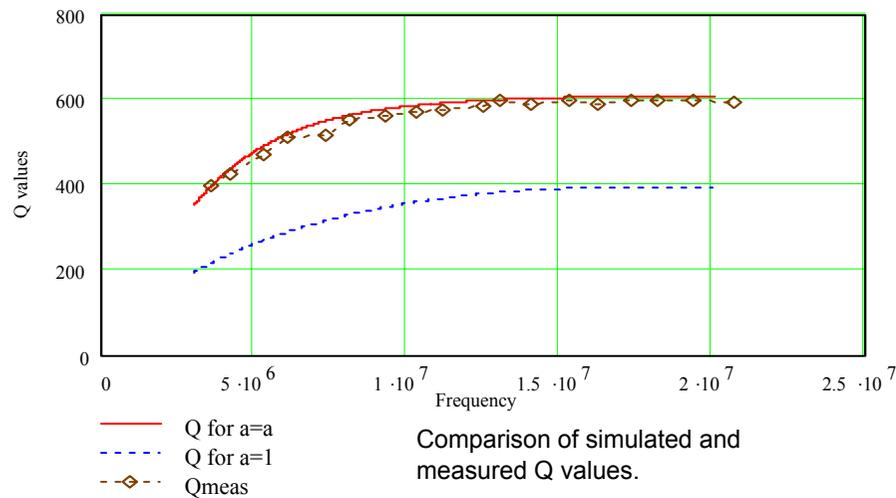
Comparison of simulated and measured Q values.
