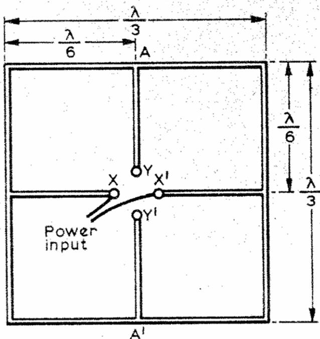
**Fig 3. Isolated inputs of the new quad element**
