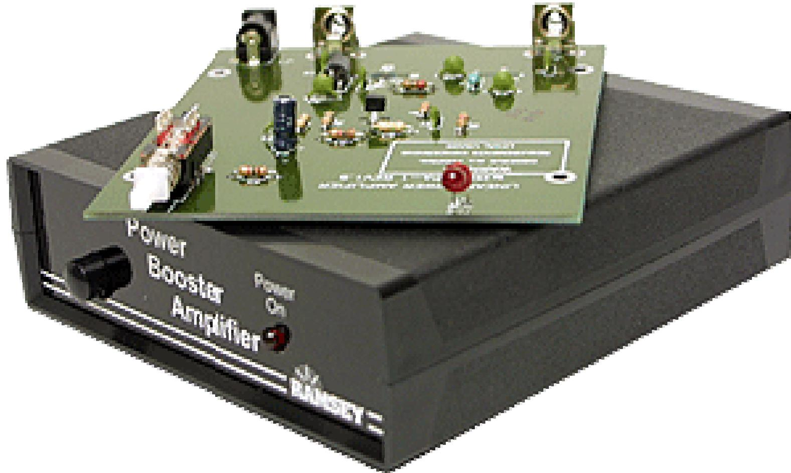
Gain of 25 – 30dB extends transmission range by > 10 times
