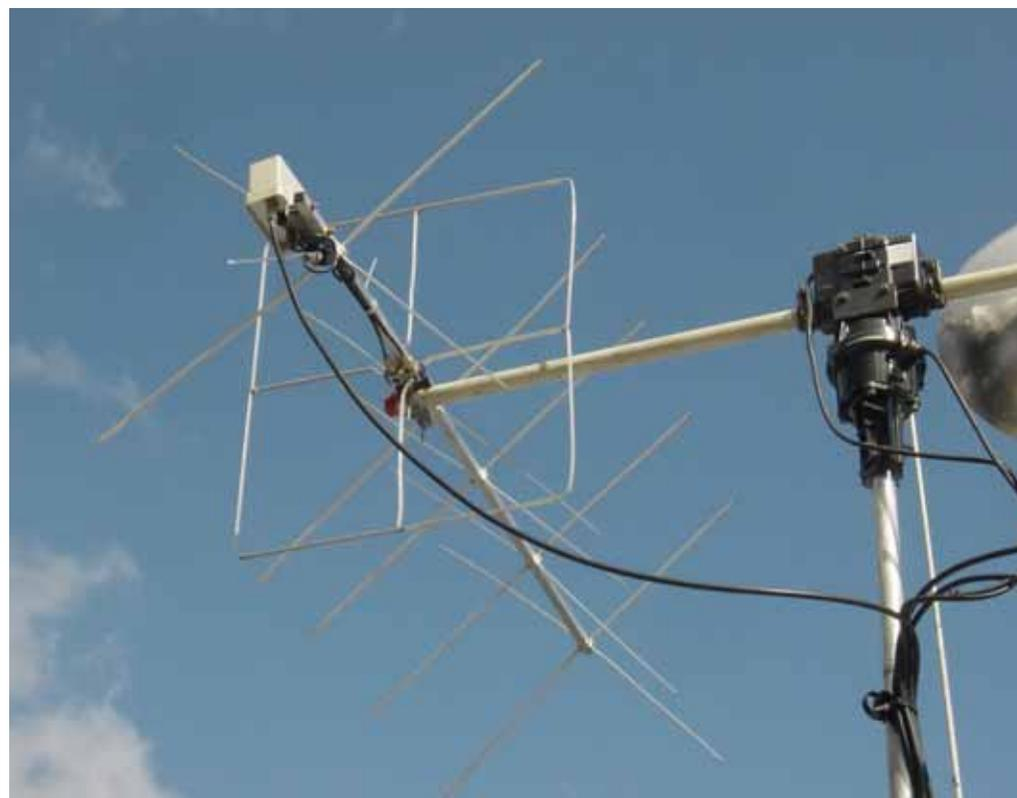
WiMo 2m Cross-polarised Antenna as on
