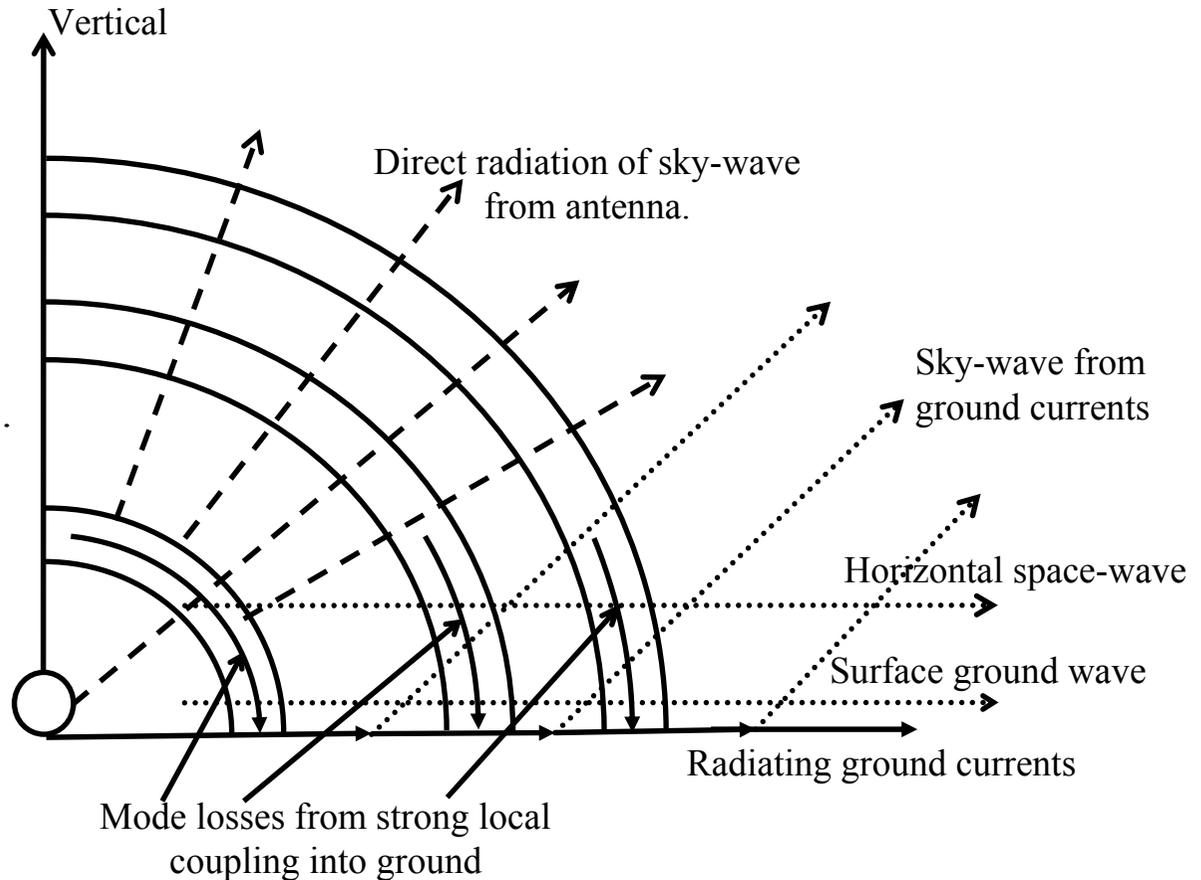
Where does the input power go? How much power couples straight into the ground under a small antenna? Does this propagate under the ground? What is the pattern and polarisation of the antenna when close to ground as compared to free space? How much surface/ground wave is launched, and of what type? Are there two or more surface wave layers.
