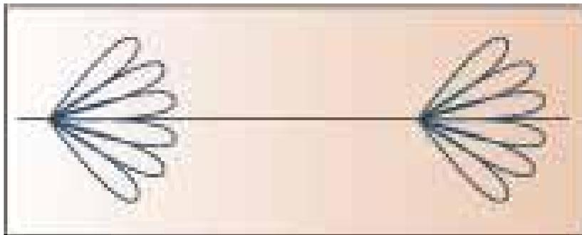
Figure 2. Radiation pattern of an antenna longer than one wavelength.
