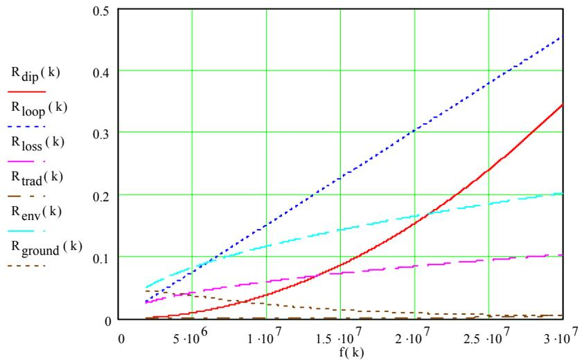
$$R_{\text{tot1}}(k) := \left( \begin{array}{l} R_{\text{loss}}(k) \dots \\ + R_{\text{ground}}(k) \dots \\ + R_{\text{loop}}(k) \dots \\ + R_{\text{env}}(k) \dots \\ + R_{\text{dip}}(k) \dots \\ + R_{\text{trad}}(k) \end{array} \right)$$
