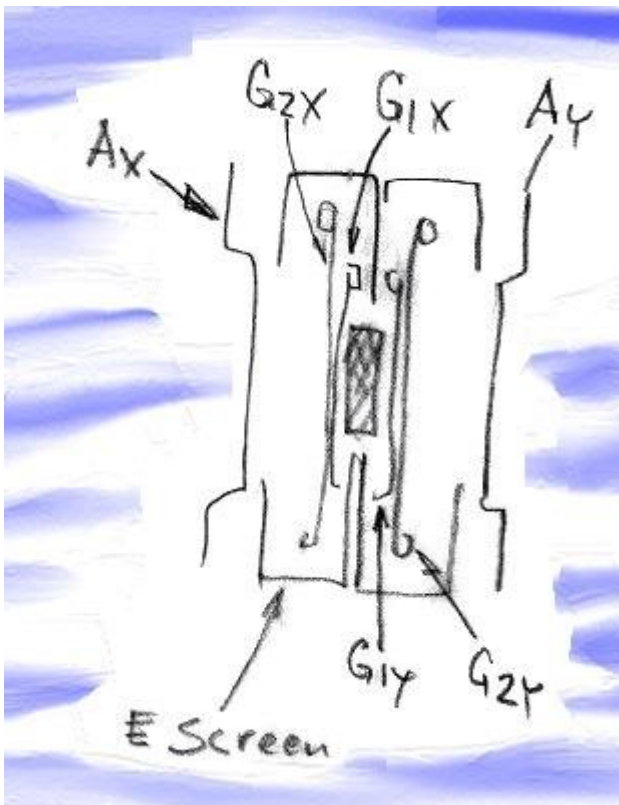
Picture 4 Sargrove's UA-55 tube had a common heater (55 V 100 mA) and cathode. The control grid, the braking grid and anode were separate for each tube. The 9-pin base did not
