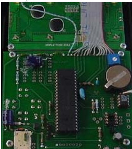
Picture 12 Two sided through coppered circuit plate with LCD and processor
