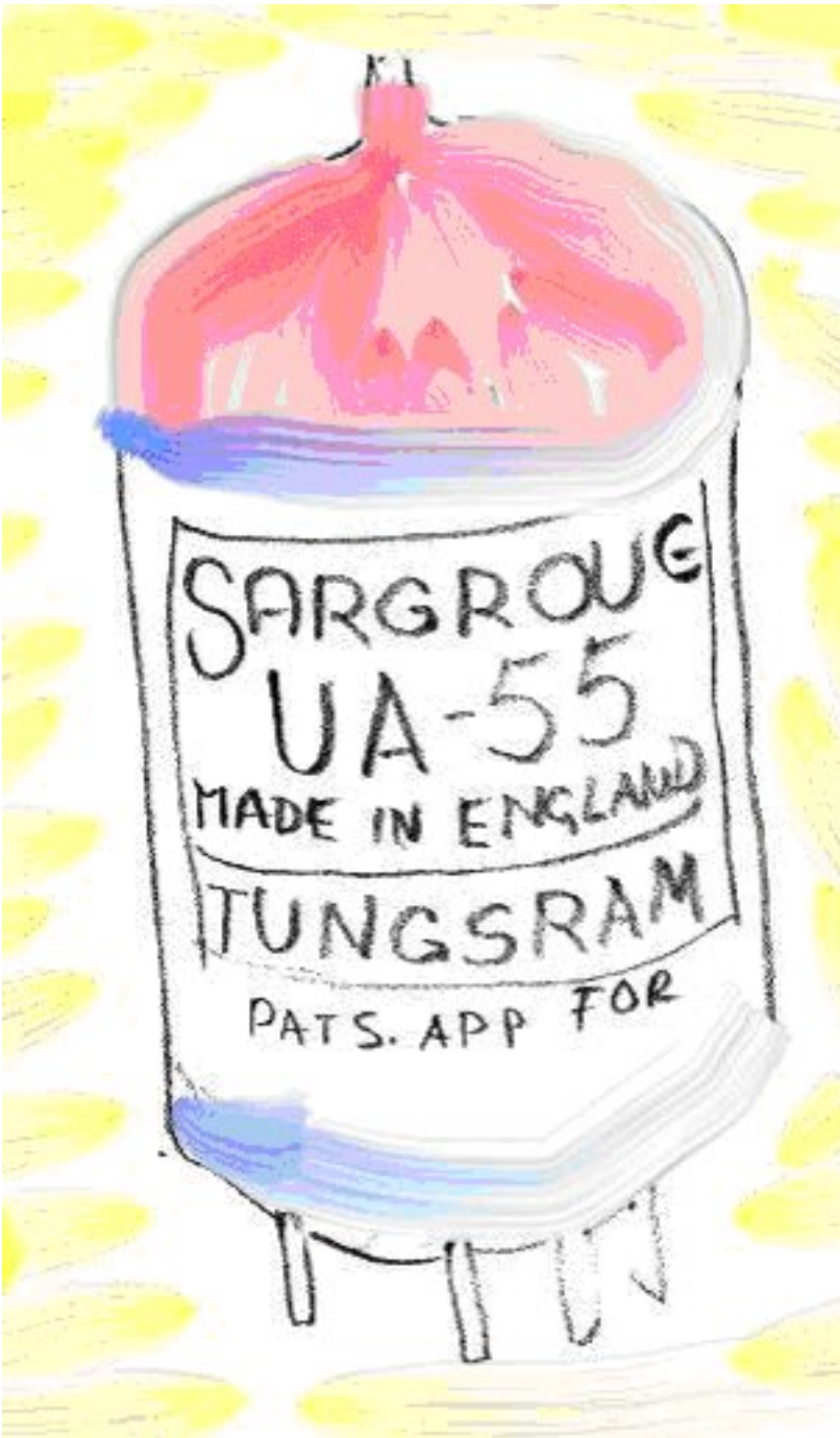
Picture 2. The basis of Sargove radio was a general tube, UA-55, witch fit every purpose sufficiently well. There were two tube functions in the same envelope.
