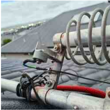
Replacement of the 30m, 67pF doorknob capacitor with a 68pF and the modified mounting.
