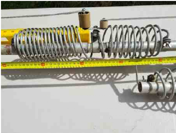
80/40m assembly, Doorknob Capacitors (left 200pF/80, right 67pF/40m)
