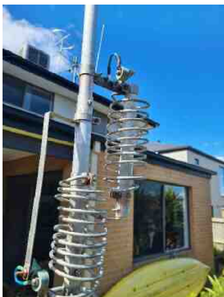
Picture above the 40m and 30m assembly with stress relieve for the two identical doorknob capacitors.
