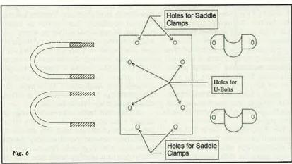
The halo is now basically finished. All that remains is to test it (and make any necessary adjustments). To do this the halo should be mounted over the car. I have mine mounted as high and as central as I can, using a roof rack bar. A basic bracket can be made from 4mm aluminium plate, 20mm plumbers saddle clamps, and two suitably sized U-bolts. This is up to you, but Figure 6 is a suggestion.
