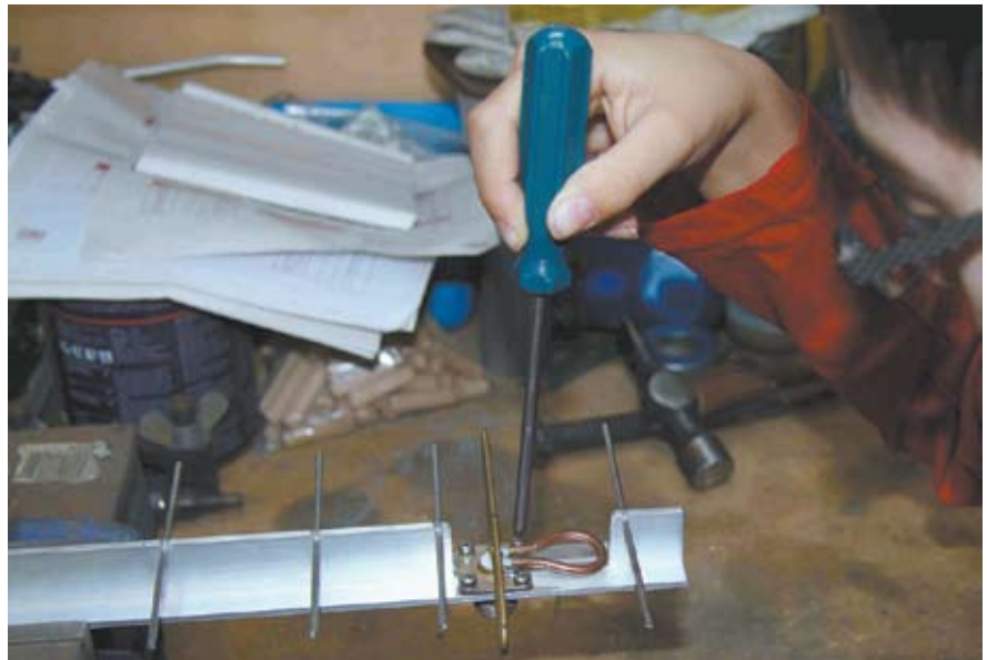
Photo 3: Fitting the Driven Element Assembly
