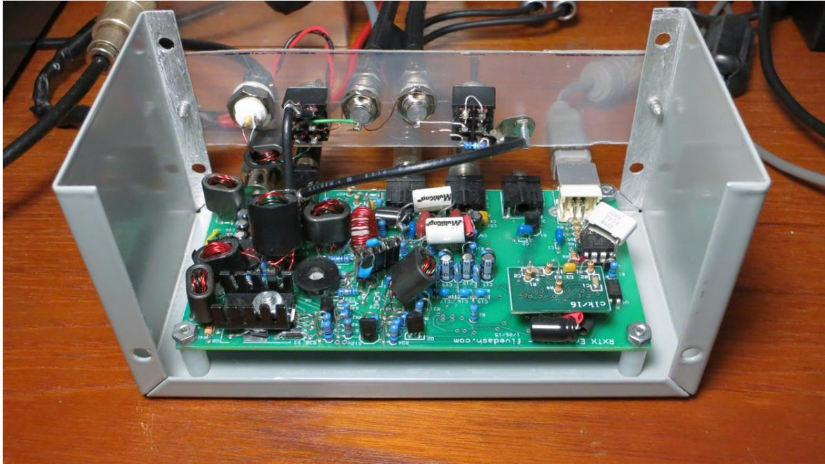
I replaced the RX attenuator plug-in (Note 5) with a plug that has two mini-coax cables. The cables go to a panel that has: first, a switch to select either the line from the T/R circuit (for the TX antenna) or an RX antenna coax jack; next, a pair of coax jacks for either a jumper cable or for a BPF or HPF; next, a switch for a 20 dB attenuator; finally, the coax cable to go back to the plug to connect to the RX mixer input transformer.
