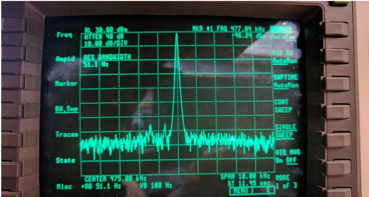
Photo 3. 1830 KHz. All spurious signals, including the image, within +/- 5 kHz of the main signal, were at least -60 dBc. The LO leak through here was -55 dBc.
