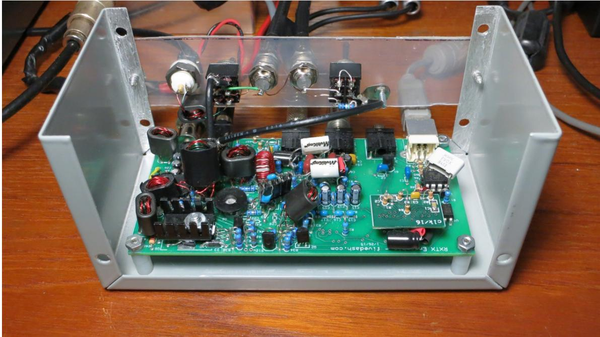
I replaced the RX attenuator plug-in (Note 5) with a plug that has two mini-coax cables. The cables go to a panel that has: first, a switch to select either the line from the T/R circuit (for the TX antenna) or an RX antenna coax jack; next, a pair of coax jacks for either a jumper cable or for a BPF or HPF; next, a switch for a 20 dB attenuator; finally, the coax cable to go back to the plug to connect to the RX mixer input transformer.
