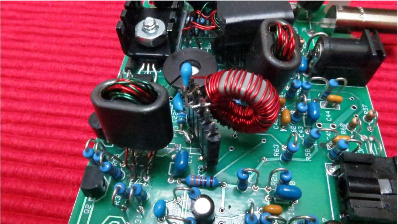
Close-up showing the plug-in TX mixer low pass filter
