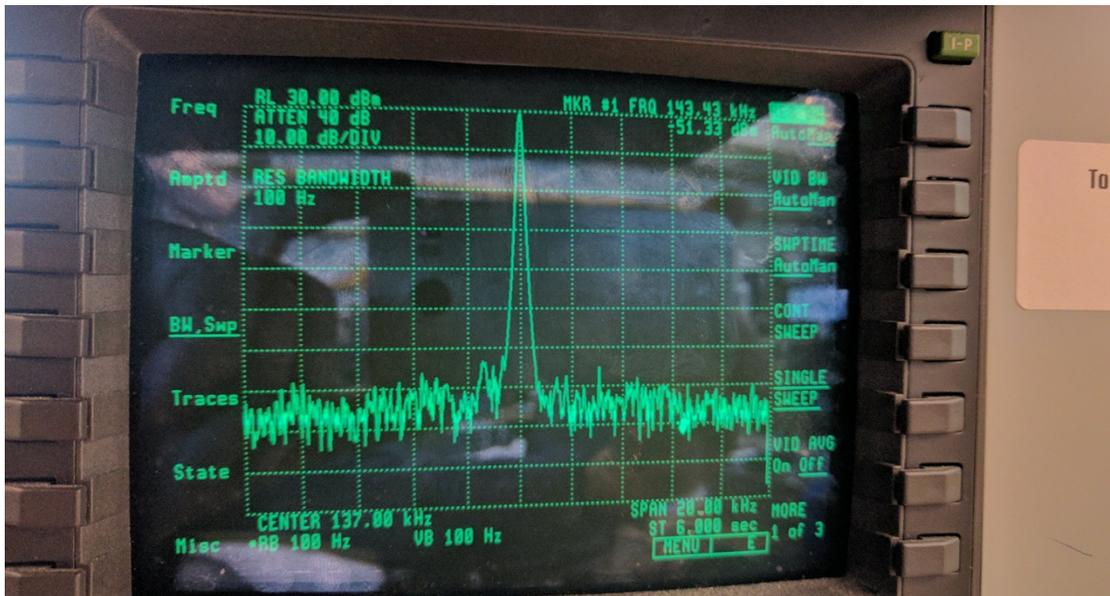
Photo 2. Output 475 kHz. All spurious signals, including the LO and image, within +/- 5 kHz of the main signal, were at least -60 dBc.
